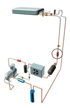
**DCY Range** Anti-acid filter driers for the filtering and drying of refrigerants and acid neutralization for liquid lines of refrigerating and air conditioning installations. Great drying and acid neutralization capacity at all temperatures. Maximal working pressure 46 bar. Filter driers sizes that ensure interchangeability with most products of the market. Installation possible in all positions.
