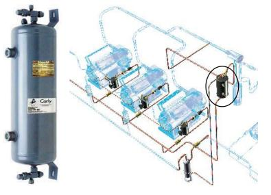
**HCYR Range** Oil receivers for storage of the oil reparated from the refrigerant by the oil separator(s) of refrigerating and air conditioning installations. This oil is then re-distributed to the compressor sumps, by means of LEVOIL mechanical or electronic oil level regulators.
