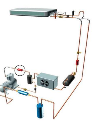
SCY RANGE - Discharge line mufflers - 64 Bar (928 psig) - CO<sub>2</sub> Subcritical
