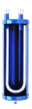
LCY Range Suction line accumlators for the elimination of risks linked to the return of refrigerant in its liquid phase and to the massive oil intake at compressor's suction of refrigerating and air conditioning installations.
